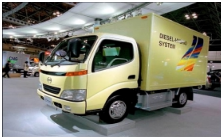
Figure 5.– Toyota’s Diesel Electric Hybrid Delivery Van
